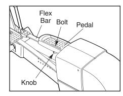
the pedal. Next, push the bolt upward, slide the pedal forward or backward to the desired position, and then retighten the knob. Make sure that both pedals are in the same position.
